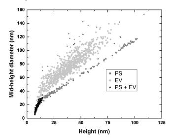
**Figure 6.** Correlation diagram between the mid-height diameter and the height of PS nanobeads and EV codeposited on poly-Llysine modified mica. The data are extracted from a unique  $20 \times 20 \ \mu\text{m}^2$  AFM image (1163 detected particles). Data represented on the graph by (+) are rejected from the analysis.
