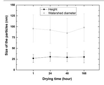
**Figure 4.** Evolution of the size (mean values) of the EV with the drying time of the sample at room temperature. Error bars represent the standard deviation calculated from 70 to 100 detected particles.
