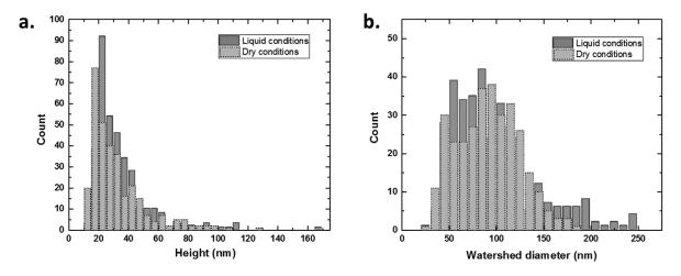
Figure 3. Size distributions of the height (a) and the watershed diameter (b) of EV measured under liquid and dry conditions. The data were obtained from the analysis of around twenty  $10 \times 10 \ \mu m^2$  AFM images.
