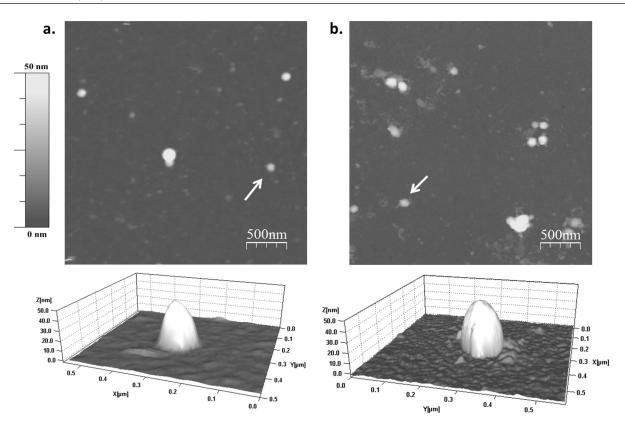
**Figure 2.**  $3 \times 3 \mu m^2$  tapping-mode AFM images of the topography of erythrocyte-derived EV immobilized on antibody-modified mica. Imaging was performed in PBS solution (a) and under dry conditions (b) at room temperature. EV appear as circular light grey particles on both images. Enlarged 3D views of the EV indicated by white arrows are presented below respective images. The *z* scale of the 3D views have been magnified to improve visualization.
