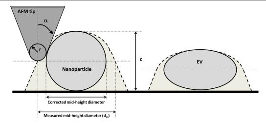
**Figure 5.** Schematic representation of the tip convolution effect on a spherical nanoparticle and an ellipsoidal EV. The AFM tip is modeled by a right circular cone with a half opening angle  $\alpha$  and a sphere of radius *r* at the apex. Diameters of the particles are determined at mid-height.
